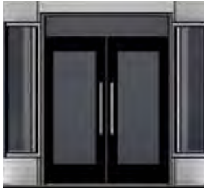
ALL ENTRANCE DOORS SHOULD BE PAINTED BLACK, WITH INDUSTRIAL TALL UNPOLISHED METAL HANDLES.
